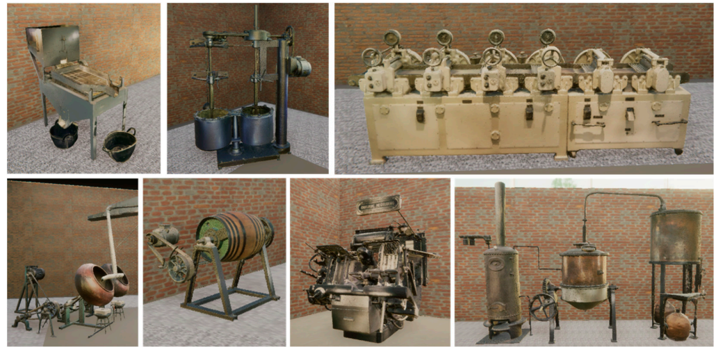
Figure 14. All the machines that were scanned and reconstructed as 3D models for the virtual factory. At the top, from left to right: Sifting machine, blending machine, and cutting machine. At the bottom, from left to right: Candy machine, revolving cylinder, printing machine, and distillation machine.
